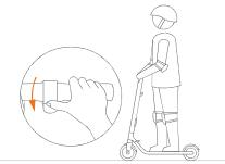
Put your other foot on the footrest to keep both feet stable. Press the throttle on right hand to speed up when you are balanced.
